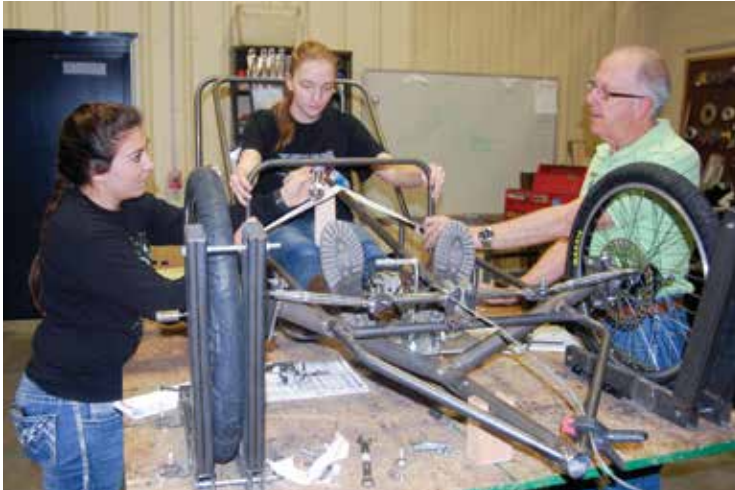
Top Left: Karlee Logan, MacKayla Koehn, and Chuck Ellis work on adjusting the steering column and the foot controls so the car fits MacKayla, who will drive the electric car in the upcoming races.
